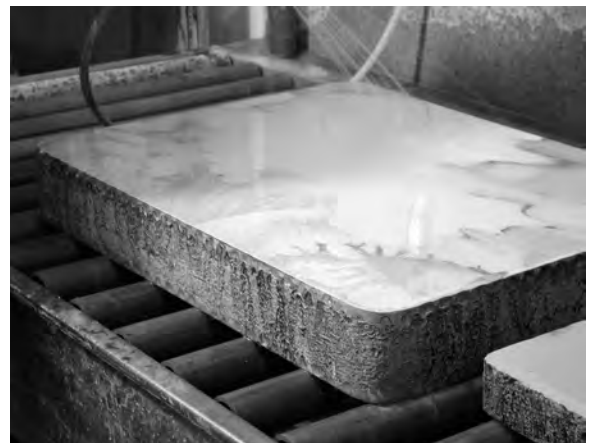
When grit becomes sticky and hard to move, wash off with water and start again with fresh grit.
