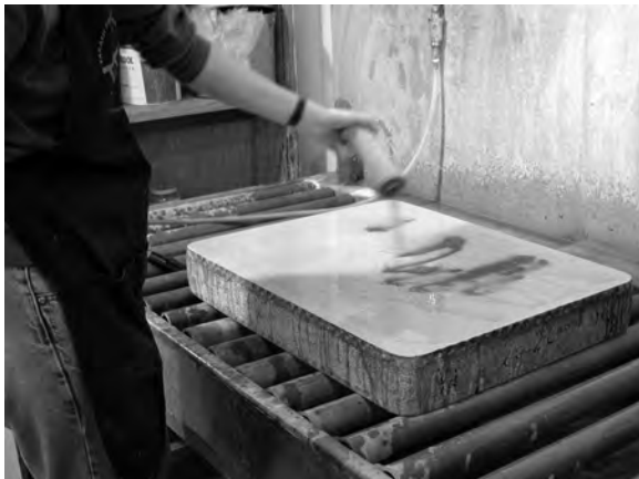
Sprinkle 100 grit on the wet stone.
