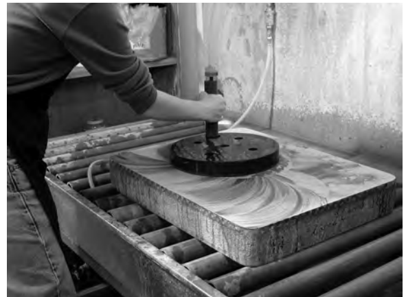
Grain using levigator 3x with 100 grit or until the 'ghost image' is gone.
