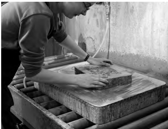
Or, grain using a flat stone, then grain 3x with 150 grit and 2x with 220 grit.
